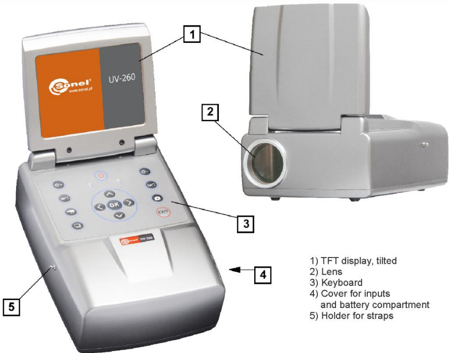
Fig. 11. Parts of Camera UV-260.
