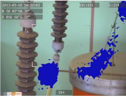
Fig. 3, 4. Corona discharge in laboratory conditions.
