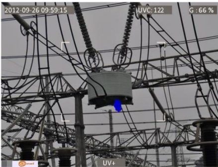
Fig. 5-8. Corona discharge in real power grids.
