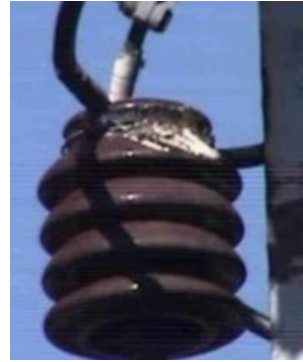
Fig. 9, 10. Corona discharge and its effects.
